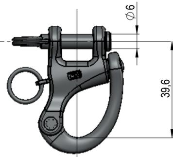
Mousqueton  $\varnothing$ 6 /  $\varnothing$ 6 Snapshackle
